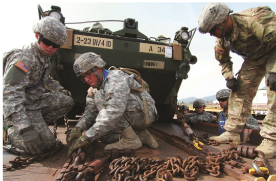
Soldiers secure a Stryker vehicle to a rail car during rail load operations. (U.S. Army photo)
