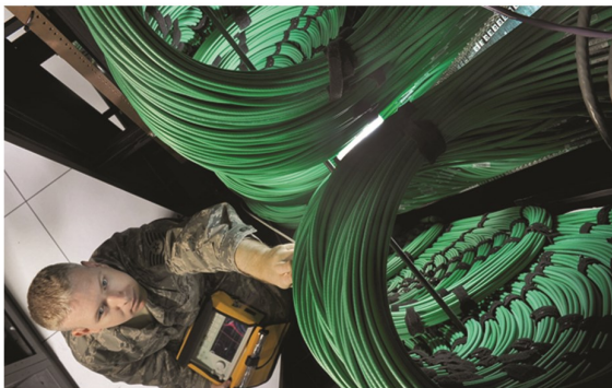
A U.S. Air Force TSgt uses a spectrum analyzer to check network routers. (U.S. Air Force photo)
