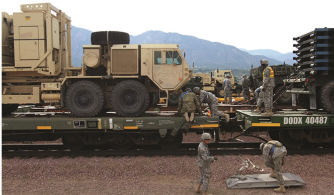
Soldiers of the 1st Stryker Brigade Combat Team, work together to secure vehicles to rail cars with chains during rail load operations for deployment. (U.S. Army photo)
