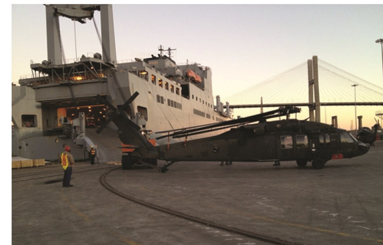
U.S. Military Sealift Command Personnel load an Army Helicopter on a large, medium-speed, roll-on and roll-off ship. (U.S. Navy photo)
