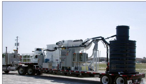
Tyndall AFB Portable Waste to Energy www.af.mil/shared/media/photodb/photos/080804-F-9999U-103.jpg
