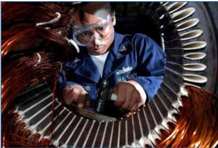
U.S. Navy Petty Officer 3rd Class Tyreek Hayward lays coil to rewind a motor in the machine shop aboard the aircraft carrier USS Nimitz in the Gulf of Oman, Nov. 9, 2009. U.S. Navy photo by Seaman Robert Winn.
