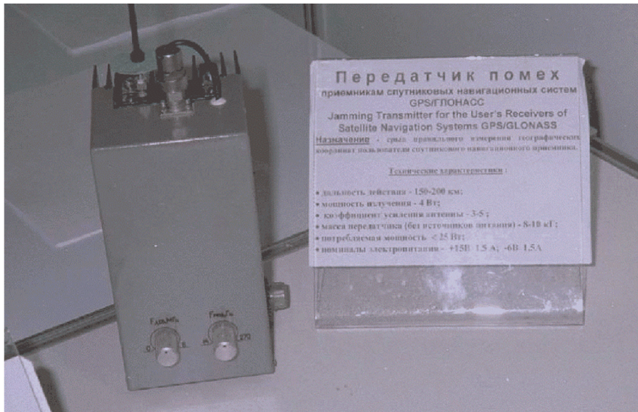
Figure 11: Russian handheld GPS jammers are available commercially worldwide.
