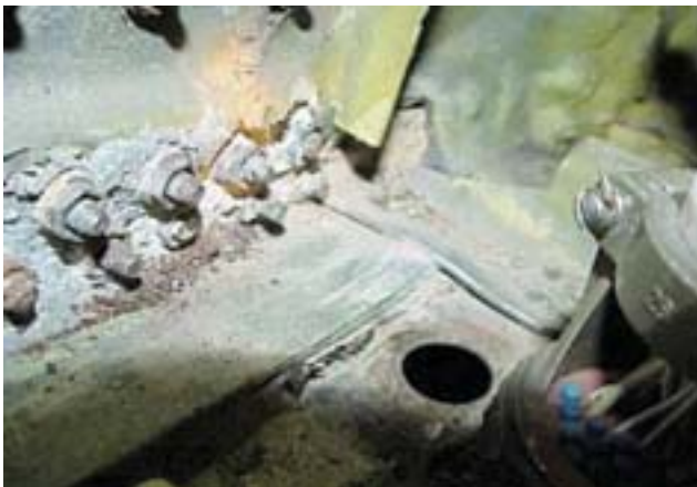
Corrosion issues such as this KC-135 engine strut (left) highlight the challenges experienced by the Air Force's aging aircraft fleet.
