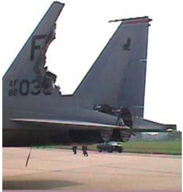
Structural failure (as seen on this F-15) remind us of the tremendous stress on our warfighting systems, many of which have exceeded their planned service life.
