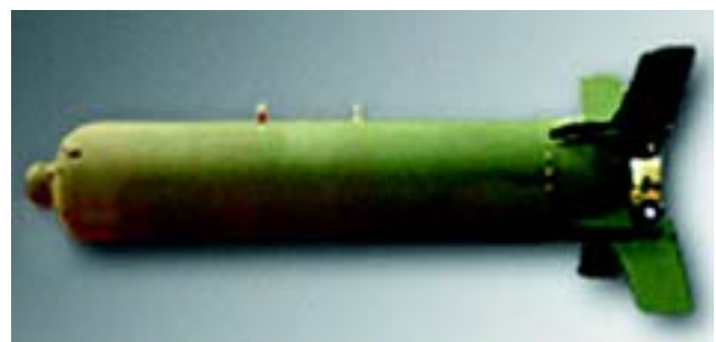
The WCMD enables combined-effects munitions to be released from high altitude — maintaining precision while limiting the risk to aircrew.
