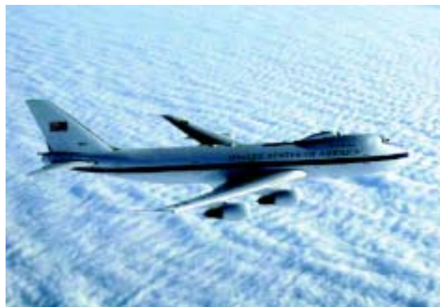
The E-4B National Airborne Operations Center (NAOC) provides the National Command Authorities a highly survivable command, control, and communications center from which to direct U.S. forces during a national emergency.
