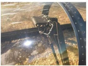
Pictures B-8: Canopy Release Bolt (CARB) properly operated
