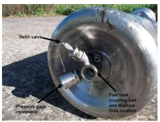
Picture B-24: Damages at AFT section of hydrazine tank. Rupture disk was found broken, however it was activated due to ground impact and not as a result of Emergency Power Unit (EPU) activation
