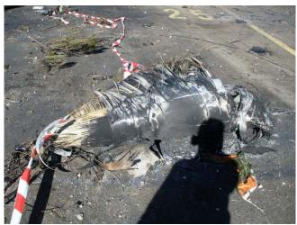
Picture B-11: The radome totally destroyed
