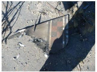
Pictures B-10: Parts of the rudder
