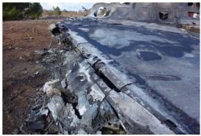
Pictures B-17: The LH wing (rear view) and close view of LH Leading Edge Flap
