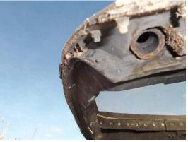
Pictures B-9: Canopy Remover Assemblies properly operated
