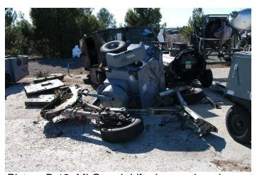
Picture B-18: MLG and drifted ground equipment
