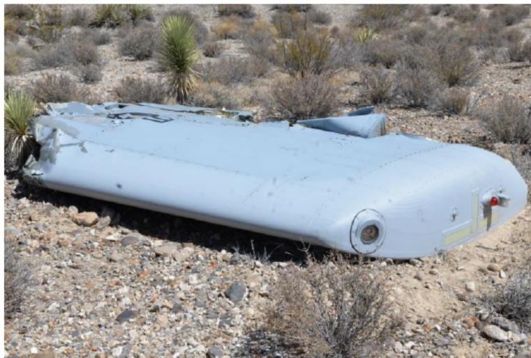
Figure 3. MA1 left wing separated in collision (Tabs S-14 and U-3)
