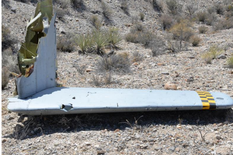
Figure 4. MA1 left vertical stabilizer separated in collision (Tabs S-16 and U-3)
