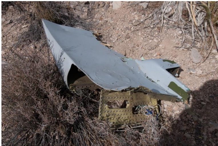
Figure 5. MA2 right wingtip separated in collision (Tab Z-3)
