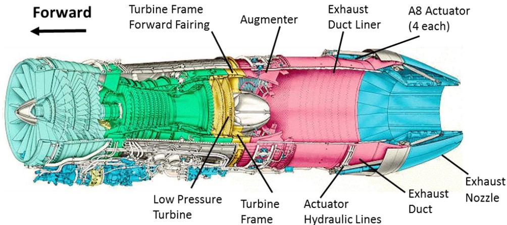
**Figure 4: F110-129 Engine Schematic (Tab CC-63)**
