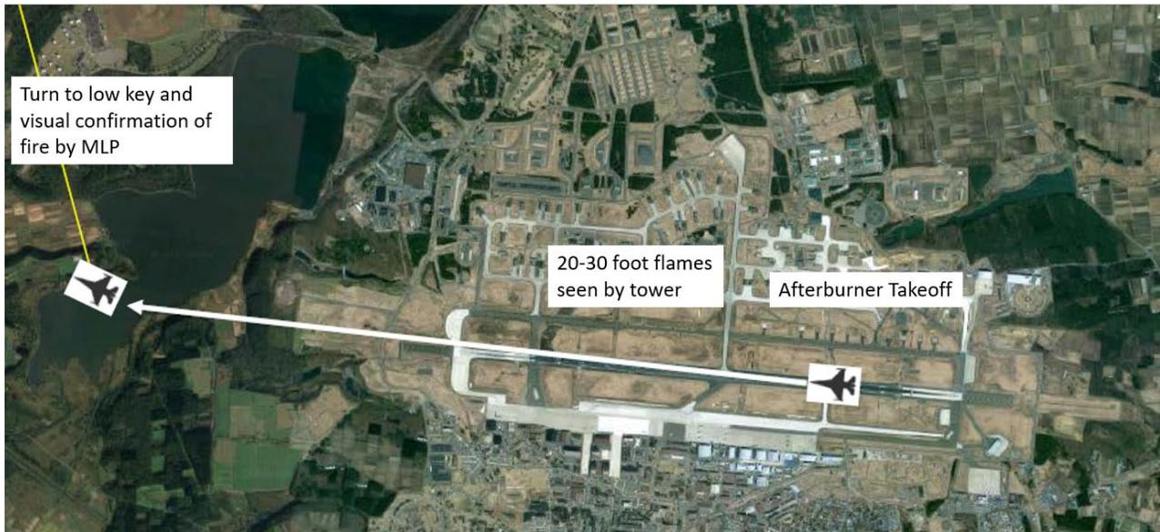
**Figure 1: Mishap Aircraft Mishap Timeline (Tab Z-31)**
