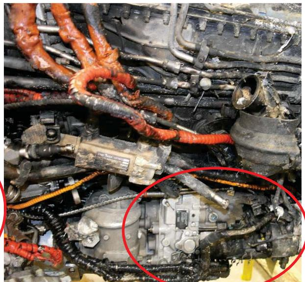
Figure 7: Main Fuel Pump/MEC Assembly (Tab J-9)
