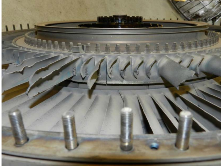
Figure 3. Stage 2 LPT Damage (Tab S-40)
