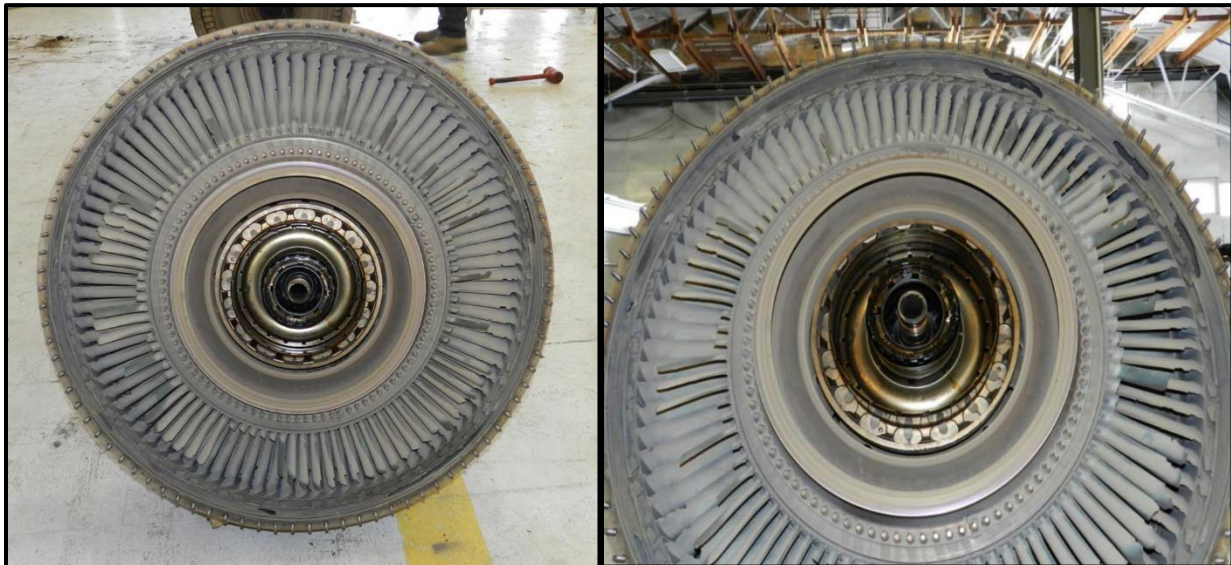
Figure 1. Stage 2 LPT Damage (Tab S-38)
