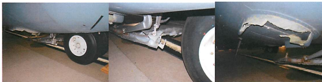
Figure 2. Mishap C-130 Gear Door and Flare Dispenser Hood
