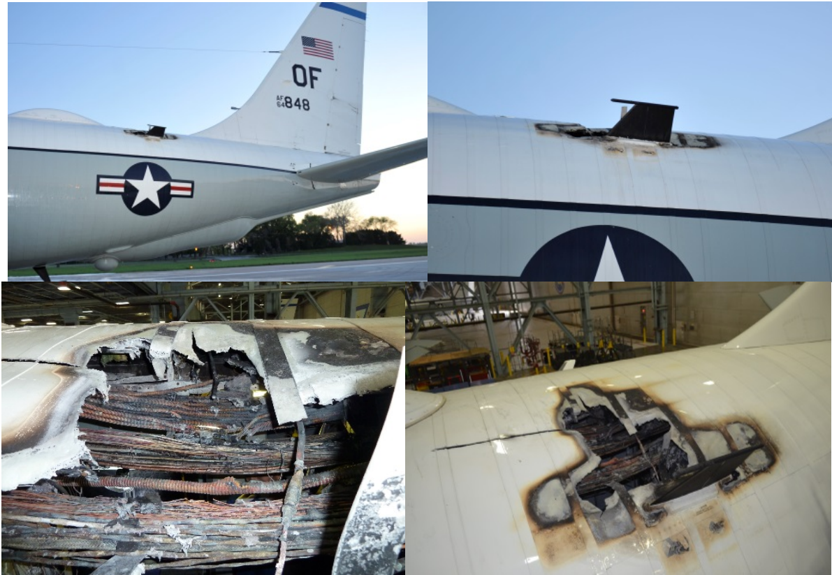
Figure 1. Damage to Fuselage (Tabs S-1.11, Z-1.4, Z-1.5, Z-1.7)
