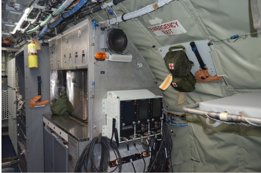
Figure 2. Undamaged Galley Area, RC-135V/W (Tab Z-1.10)
