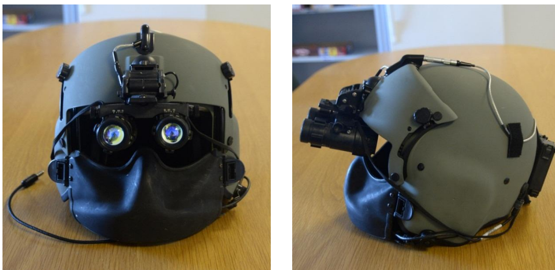
Figure 4: ANVIS-4949 Night Vision Goggles Mounted to HGU-56/P Helmet (Front and Side Views) (BB-292).
