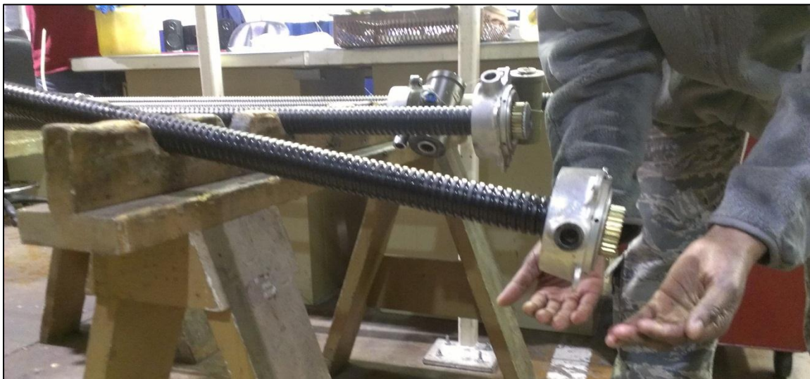
Figure 13. Drivescrew Held at Incline with Retainer Plug Missing
