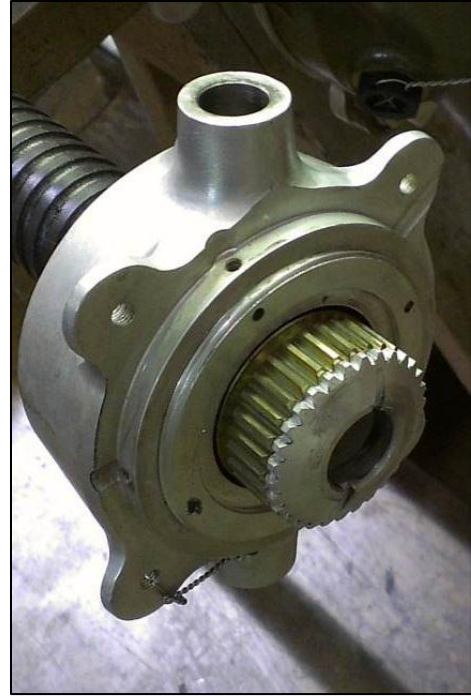
Figure 8. B-52 Flap Drivescrew Retainer Plug Installation
