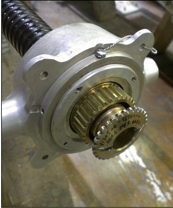
Figure 8. B-52 Flap Drivescrew Retainer Plug Installation
