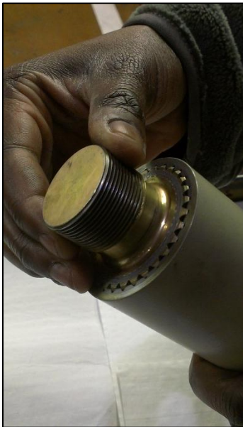
Figure 9. B-52 Flap Drivescrew Adapter Tube Assembly
