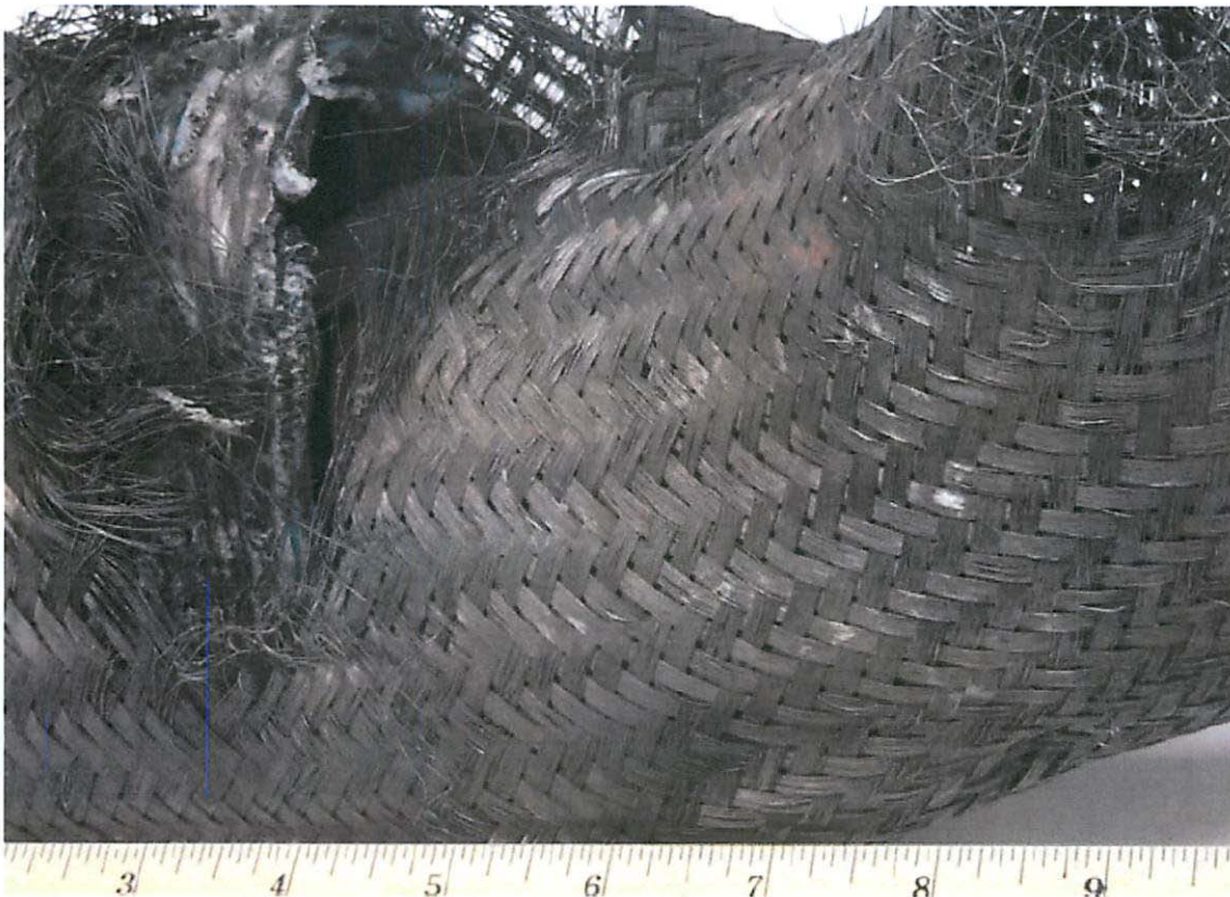
Photograph 2. Damage to 4.5-Inch Main Fuel Line (Tab J-122).
