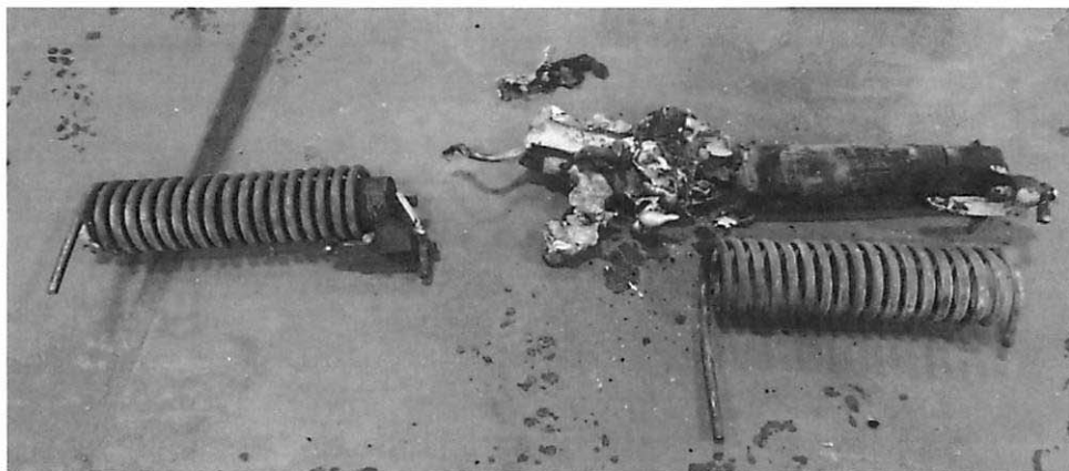
Photograph 1. Recovered Left Mandrel Spring Assemblies (Tabs GG- 3 to GG-5 and Z-22).
