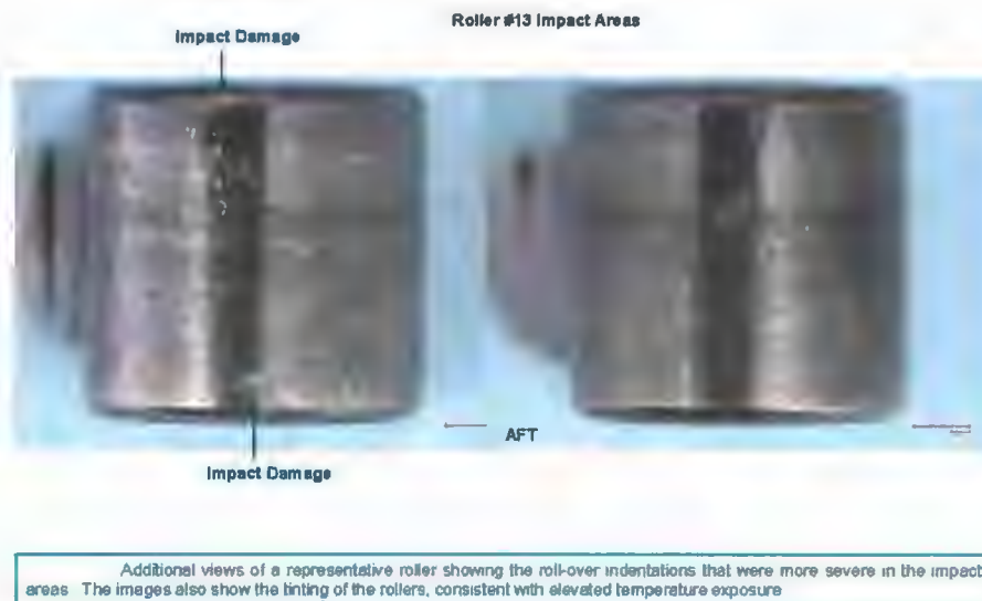
Figure 16: Roller Bearings with Indentations (Tab J-67)
