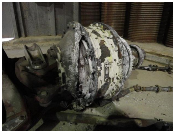
Figure 16. Main Rotor Gearbox
