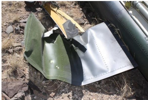
Figure 13. Crumpled Left Synchronized Elevator
