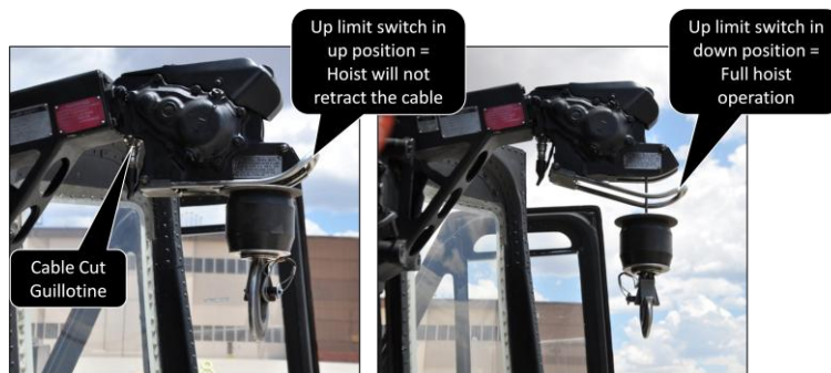
Figure 6. Hoist Up Limit Switch and Hook
