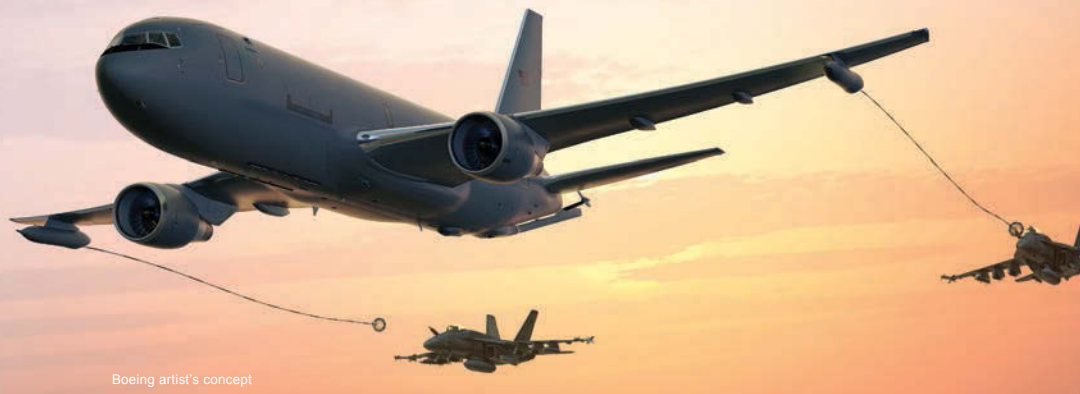
Left: The Pegasus tanker will employ both flying boom and probe-and-drogue refueling methods. Here, two US Navy Super Hornets get in place for a refill. Below left: MSgt. Luis Rodriguez-Asad, superintendent of KC-46 test operations, tries out a KC-46 boom operator demonstration at McConnell AFB, Kan.
