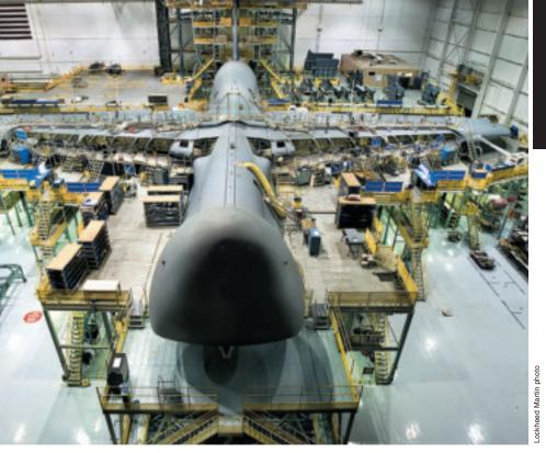
Far left: SSgt. Jason Siverling adjusts a strap on a C-17 before a drop in Southwest Asia. Left: A C-5 is transformed through re-engining and refurbishing into a C-5M Super Galaxy at a Lockheed Martin facility. Selva says the C-5M has "magnificent capability."
