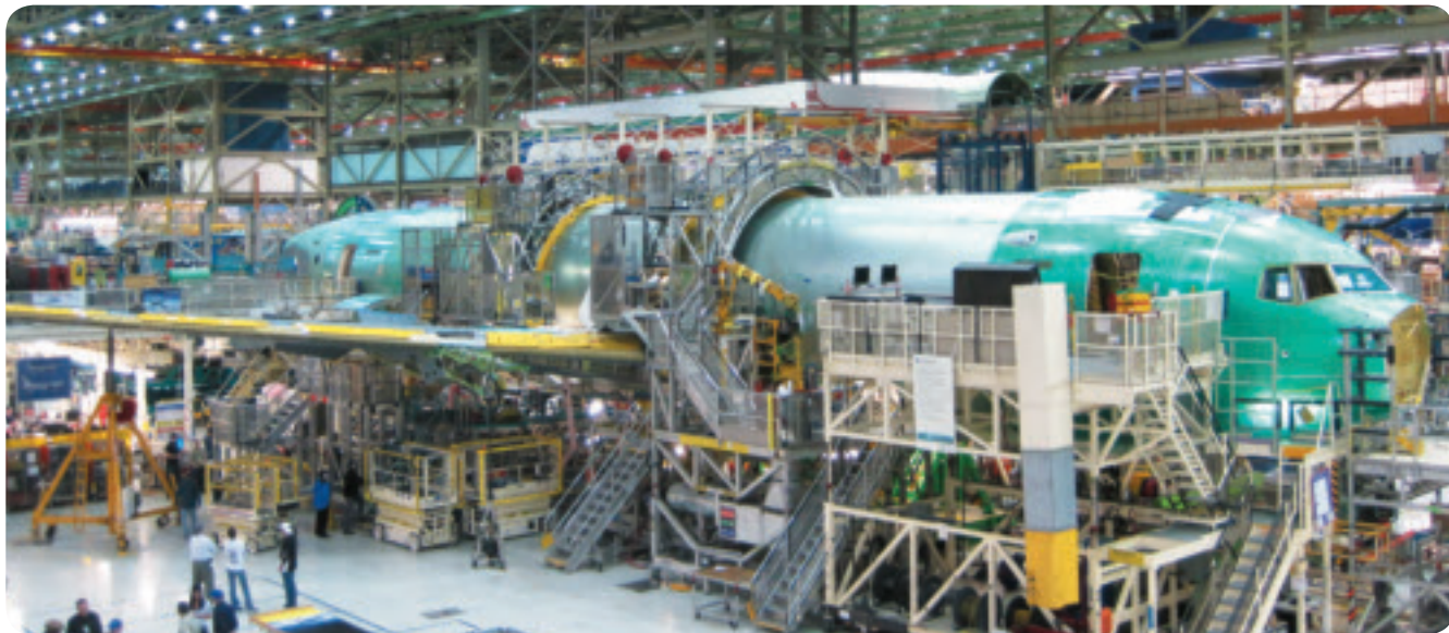
Major sections of what will be the first KC-46 are joined at Boeing's plant in Everett, Wash.
