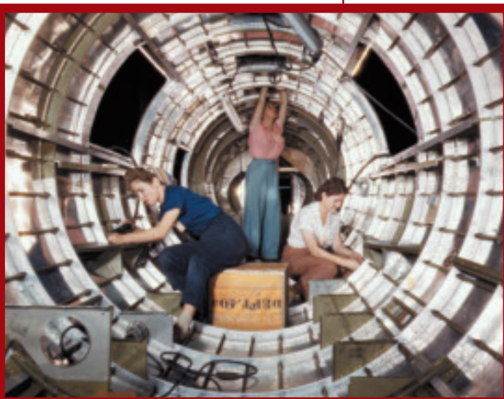
Millions of “Rosie the Riveters” entered the defense manufacturing industry. Here, women install fixtures and assemblies to a tail fuselage section of a B-17 at the Douglas Aircraft plant in Long Beach, Calif.
