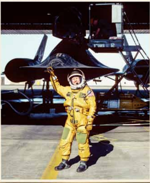
Maj. Buz Carpenter, 1st Strategic Reconnaissance Squadron, stands in front of an SR-71 at Beale AFB, Calif., circa 1979. He flew "on the periphery" of Cuba, China, and the Soviet Union. Note the fuel puddles on the ground behind him; he says maintainers at Kadena AB, Japan, wore raincoats to protect against fuel leaking down on them. Retired Col. Carpenter is a member of the Donald W. Steele Sr. Memorial Chapter, Va.
