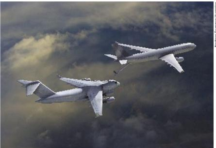
Top: A KC-767 refuels a B-52. Above: A Northrop Grumman illustration of a KC-30 refueling a C-17.
