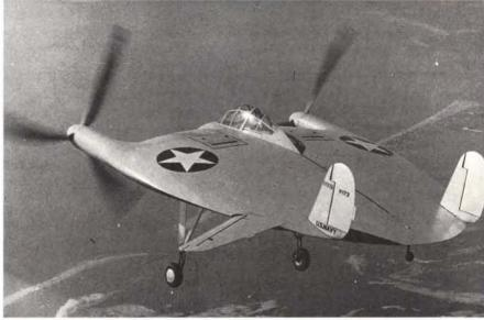
Aircraft designers sometimes use the same approach to solve different problems. The Vought V-173 "Flying Pancake" (above) owes its low-aspectratio design to a quest for reduced drag, while Lockheed Martin's F-117 (top) takes a similar shape in order to reduce radar signature.
