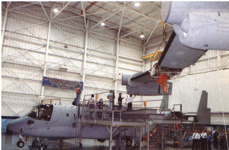
At Bell Helicopter Textron's Flight Research Center, Arlington, Tex., a crane moves the wing and nacelle structure of a V-22 Osprey into place on the aircraft's fuselage, signaling the start of final assembly. Bell Boeing officials say production of the tiltrotor aircraft is on schedule.
