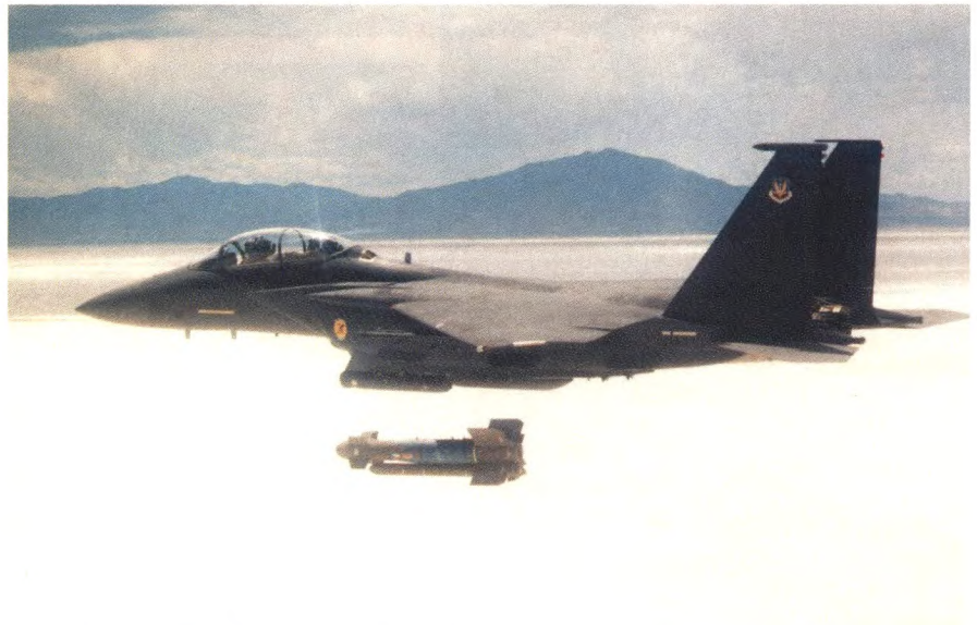
Beginning this year, Rockwell International Corp.'s AGM-130s will incorporate the latest INS/GPS autonomous guidance and infrared technology. Above, Texas Instruments conducts an operations test on an AGM-130 with an F-15E from Seymour Johnson AFB, N. C.
