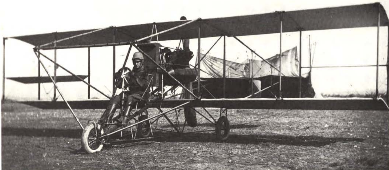
Lt. Harold Geiger in a Curtiss Pusher S. C. #8 airplane at San Diego, Calif., in 1913. Curtiss planes made use of wing-warping but employed independent ailerons for control. The Wrights' patent suits against Glenn Curtiss dragged on for eight years, outlasting their ownership of the Wright Co. and its patents and outlasting Wilbur himself.
