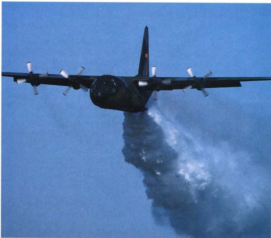
The crews generally drop all 3,000 gallons of retardant on a fire in one six-second drop, although incremental drops can be made with two of the sets. The MAFFS equipment is owned and contract-maintained by the US Forest Service.
