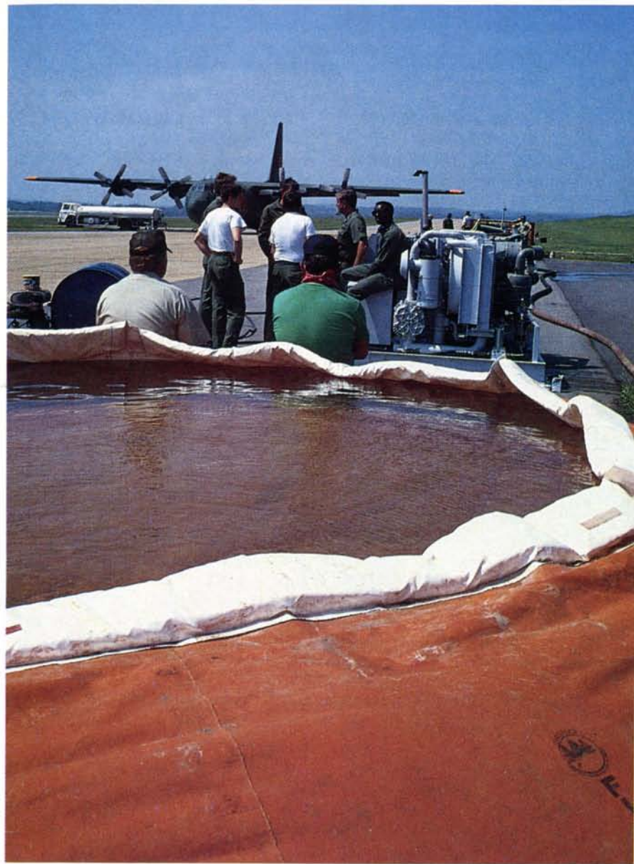
The retardant, a mixture of fertilizer, red dye, and water, is highly corrosive to the aircraft. That fact, plus the cost, are the main reasons water alone is used during training. Here, a pump crew takes a breather while one of the 145th TAG's airplanes (in the background) is refueled and refilled.
