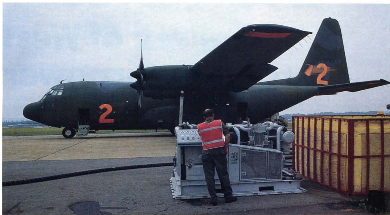
The ground crews have to pull double duty on MAFFS deployments. During the day, they man the pumps that load the aircraft with retardant or water. At night, crew members do their regular job of maintaining the C-130s. Here, a 943d TAG C-130 is refilled for another drop. The paint for the numbers and trim is mixed with soap for easier removal.
