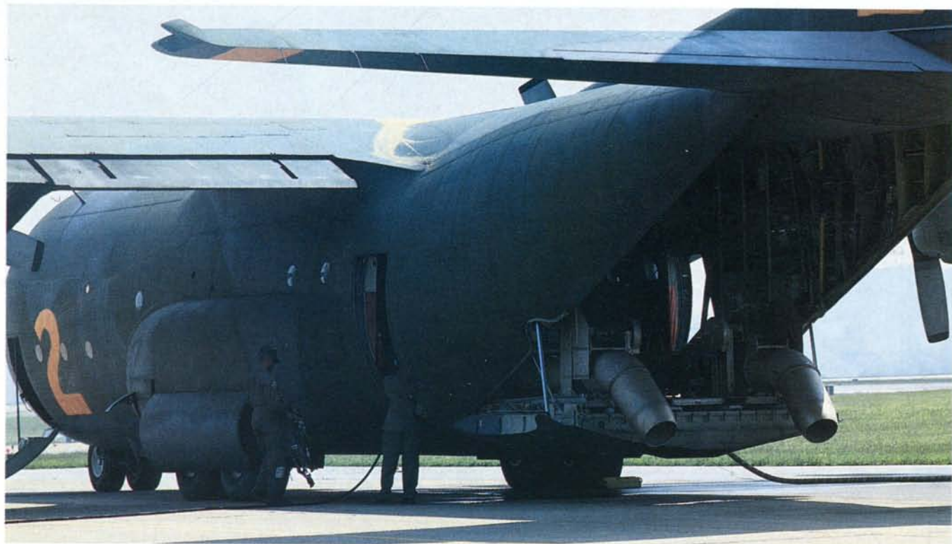
Aerial firefighting is a unique mission for four tactical airlift units. Using the palletized Modular Airborne Firefighting System, the C-130 crews can drop 3,000 gallons of retardant on a blaze. This 943d Tactical Airlift Group C-130 is being prepped for the day's practice runs near Knoxville, Tenn., earlier this year.
