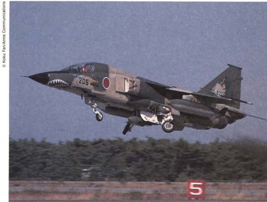
The Mitsubishi F-1, a made-in-Japan support fighter, will be replaced by advanced SX-3s in the 1990s. Deliveries of the single-seat, supersonic F-1s began in 1977. Powered by two Rolls-Royce engines, it can carry two air-to-surface missiles, 750-pound bombs, and four AIM-9 Sidewinder missiles.
