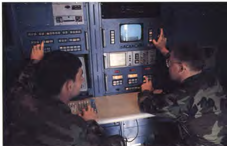
Playing the electronic “bad guys” is a role the 392d Electronic Combat Range Squadron takes very seriously. Here, Sgt. Dan McDaniels (left) and Sgt. Hoyt Hagens track a target in the AN/MSQ-T43 Modular Threat Emitter, which accurately simulates Soviet anti-aircraft artillery and surface-to-air missile radars.
