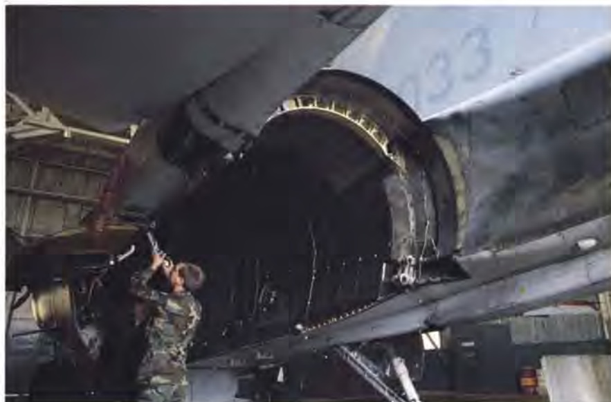
The 390th ECS at Mountain Home AFB, Idaho, represents the nonlethal side of electronic warfare—radar jamming. EF-111A crews can jam transmissions in several ways. Above, A1C John Moore and Sgt. Curtis E. Sargent prepare an EF-111 for one of the uprated TF30-P-109 engines now being fitted to the Ravens.
