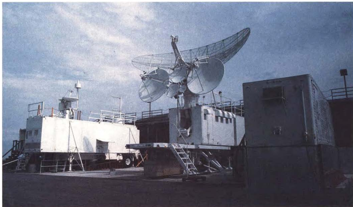
Six permanent radar bomb scoring sites, such as this one near Belle Fourche, S. D., are scattered over the fourteen low-level training routes that make up the Strategic Training Route Complex. Shown are the MUTES and TRAINS, a pair of systems that first imitate the signals of up to ninety threat radars and then record the bomber crew's reaction to those signals.
