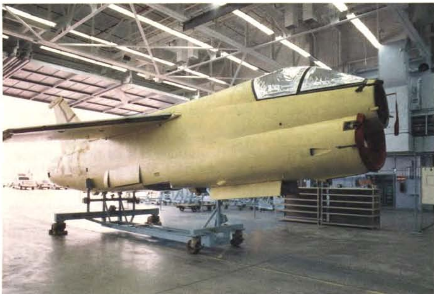
There may be a role for the A-7, shown here being modified at LTV's Texas plant for an "A-7 Plus" (YA-7F) configuration, in the AirLand Battle force of the future. Equipped with new engines, avionics improvements, and airframe modifications, the enhanced version will take part in the coming flyoff of close air support contenders.
