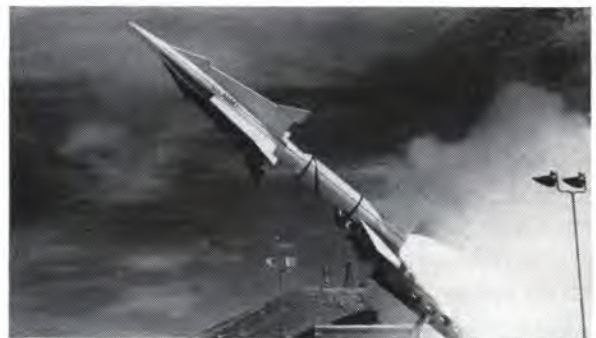
A 1960 test firing of an early model Nike-Zeus from White Sands Range, N. M., with missile sent on an unguided ballistic trajectory. AF cooperated in tests.
