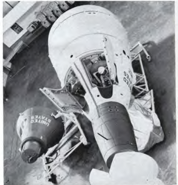
Space capsules, still not luxury sized, are growing larger, as witness this comparison between Gemini (right) and Mercury (left) on display at McDonnell Aircraft plant, St. Louis, Mo. Gemini spacecraft will weigh three tons, nearly double the Mercury craft.
