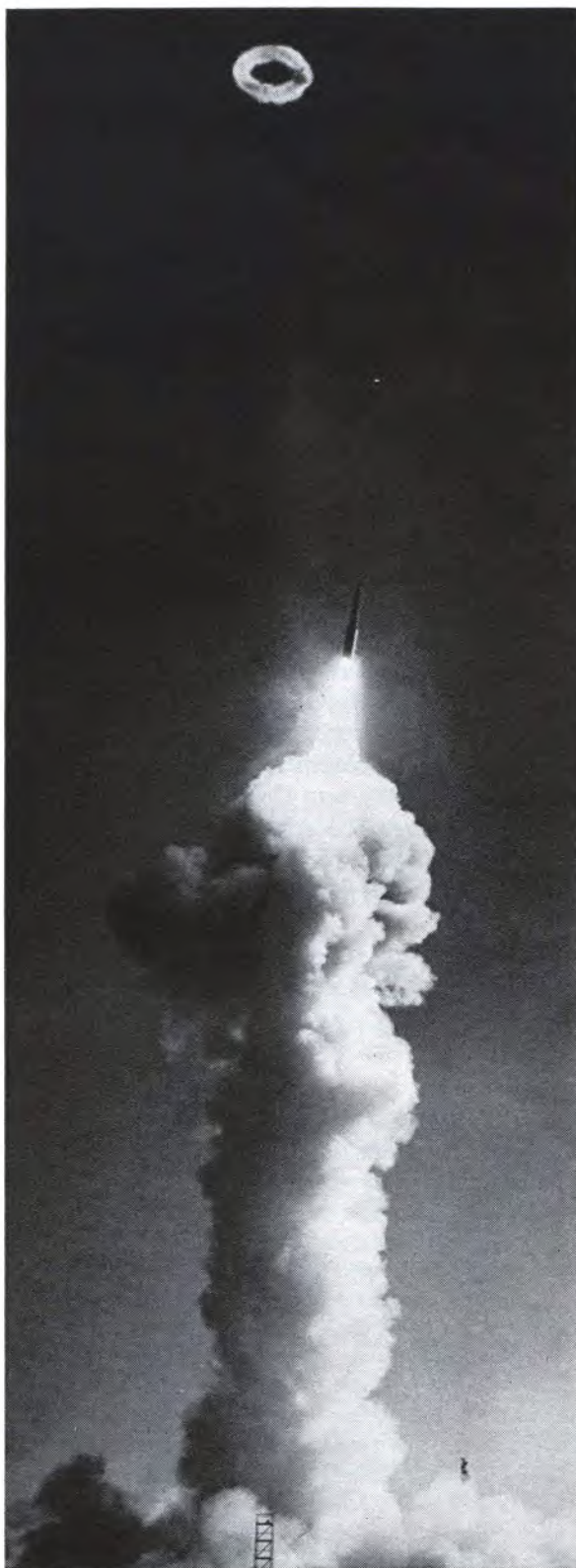
Smoke ring created by silo launch precedes Minuteman missile as it takes off on 5,000-mile flight. Concept of concurrency development was epitomized in three-stage solid-propellant Minuteman; all stages and all systems worked perfectly in its first launch.
