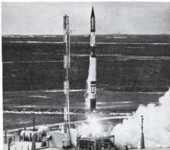
Low-budget Vanguard IGY program lagged behind Soviet effort, was dogged with failures. This launch June 22, 1959, from Cape Canaveral, failed to orbit as did all but three Vanguards. Policy choice to use nonmilitary boosters for IGY was unfortunate.
