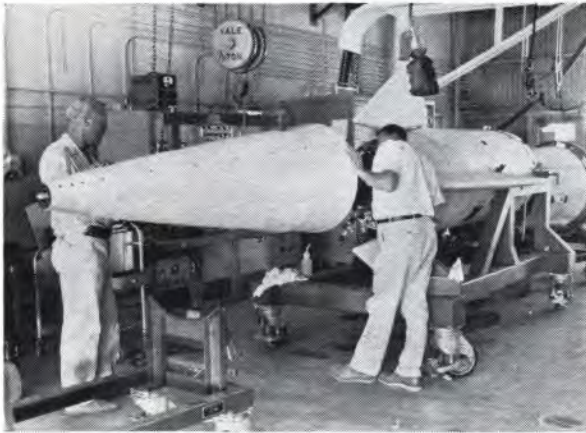
Handle with care is watchword as technicians at White Sands Missile Range, N. M., join component parts of the Nike-Zeus nose cone in the missile assembly building prior to a research firing. Each section is handled separately and joined before firing.
