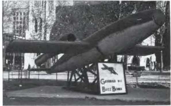
First guided missile to be widely used in wartime was the German V-1 pulsejet buzz bomb, shown here in a postwar US display. Before the end of World War II, AAF tried to copy it for use against Germany and Japan but failed to build a flyable model in time.
