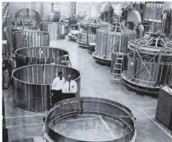
Thin welded bands of gleaming stainless steel are formed into tanks for the Atlas ballistic missile at General Dynamics/Convair plant in San Diego, Calif. Collapsible rings kept sections in circular form until missile was assembled and pressurized.
