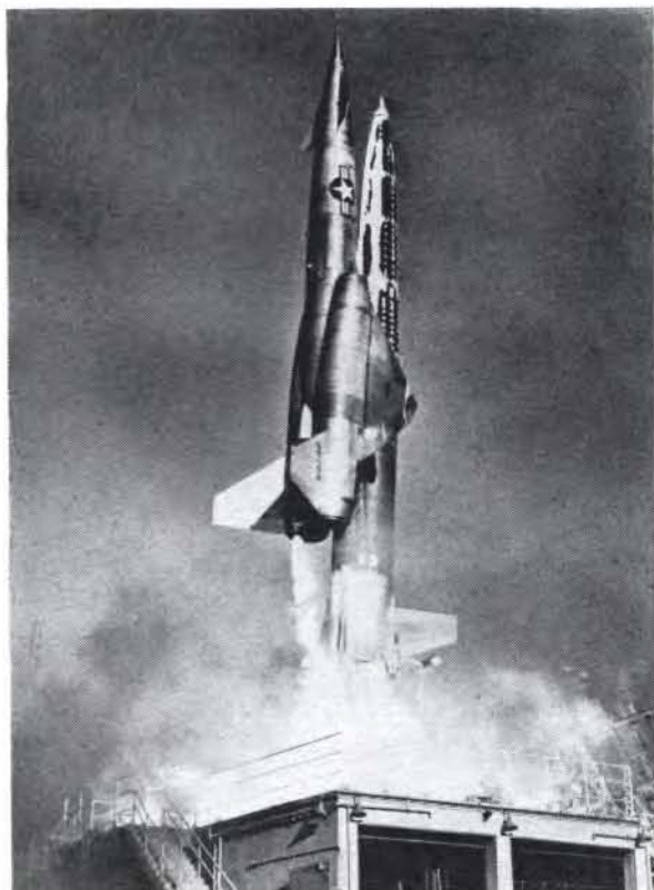
North American Navaho, riding piggyback on its rocket booster in this test flight, was to be a supersonic air-breathing missile of intercontinental range. Though it never reached production, its rocket booster is forerunner of many current USAF missiles.
