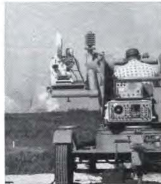
Indicative of new complex of industrial and military resources developed to meet missile program's research and testing requirements is this tracking camera recording a Titan II launch at Cape Kennedy.
