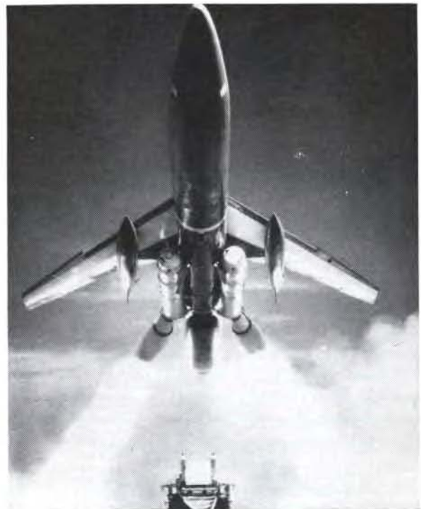
Northrop Snark, shown here in 1958 test flight from Cape Canaveral, was first US guided missile with intercontinental range. It never achieved design specifications, but broadened the base of the technology.
