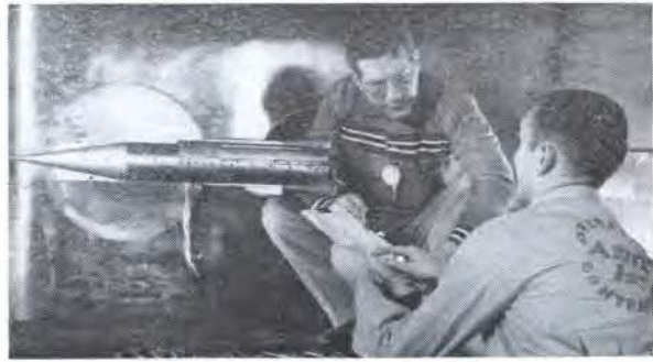
Technicians mount 1/30th scale model of Atlas in von Kármán gas dynamics facility at AEDC in preparing for test of missile configuration and propulsion.
