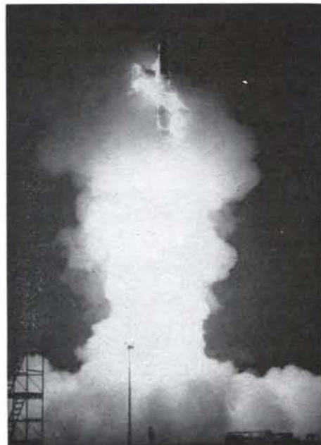
Minuteman encircled by flame at left illustrates rough conditions of silo firings. But such firings have proved to be much easier than was predicted in many quarters.
