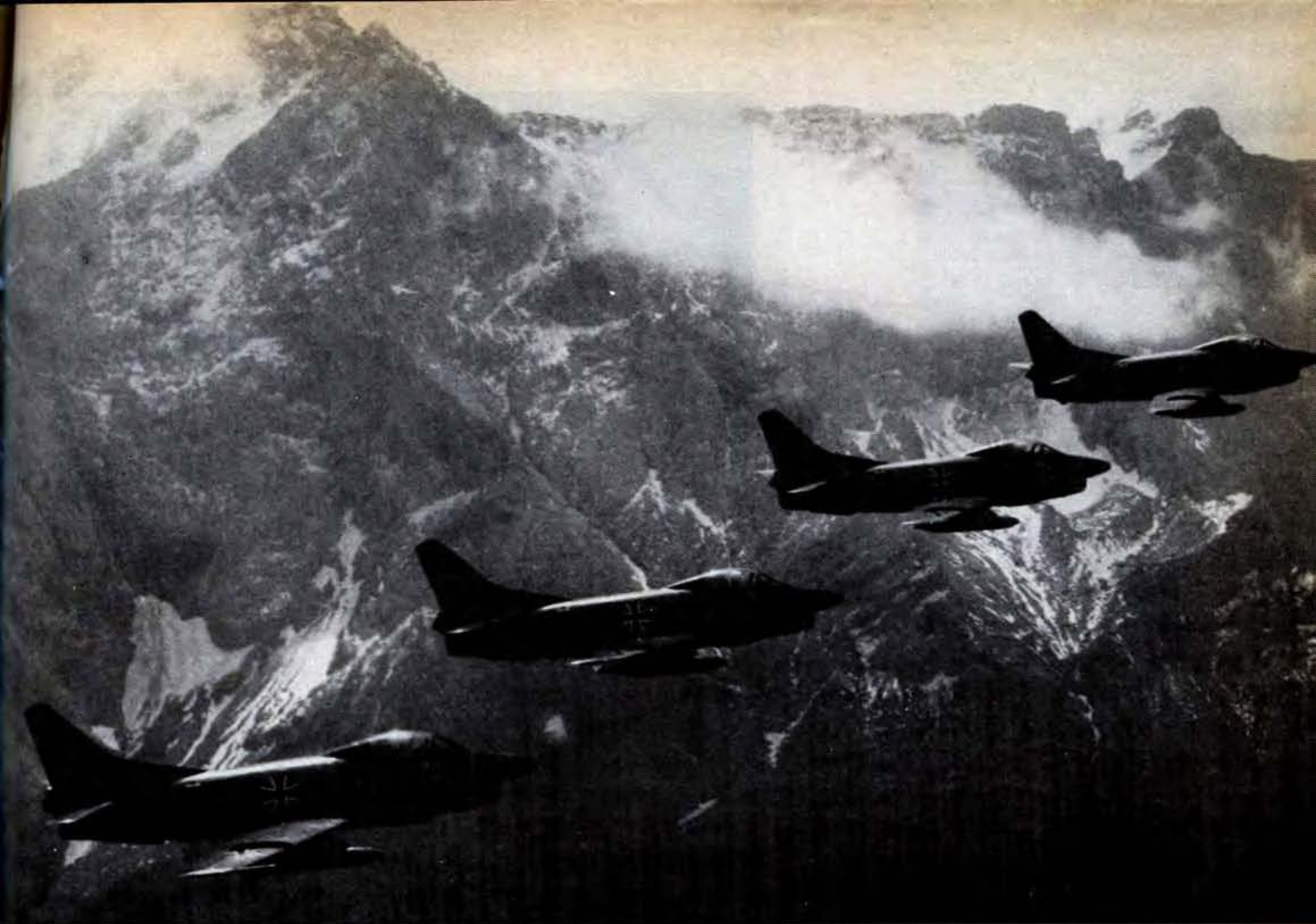
Four of the Luftwaffe's little Fiat G.91 fighter-bombers fly through cloud-covered Alps. The subsonic G.91, now obsolescent, resulted from NATO design competition. It can take off from grass fields, is also used for close support.
