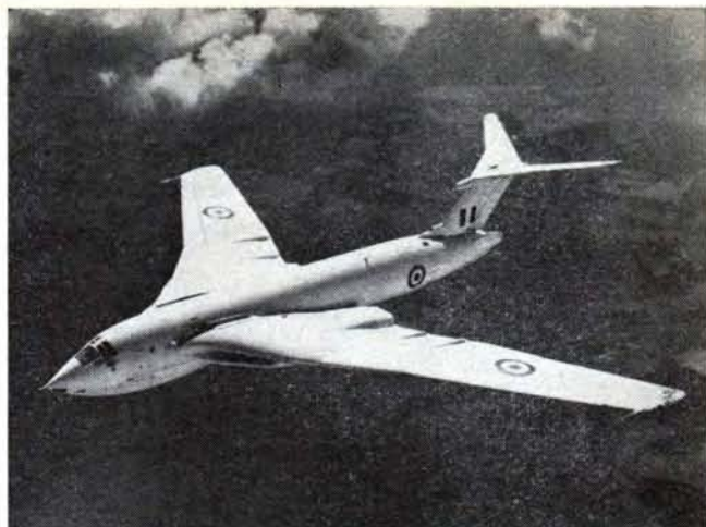
Biggest and heaviest of the V-bombers is Victor, characterized by crescent-shaped wing. Like Vulcan, it carries either nuclear or conventional bombs or Blue Steel missile.
