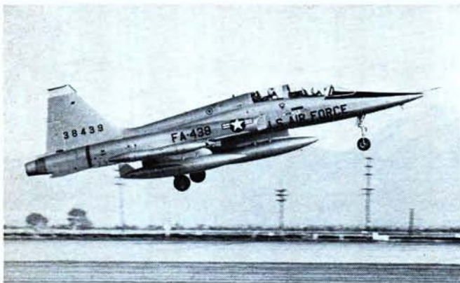
First F-5B takes off for delivery to TAC last April. Structure is conventional semimonocoque with stressed skin, longerons, and frames. Seventy-five percent of the F-5B structure is common to the F-5A and the T-38. Most major systems are more than 80 percent common on the aircraft.
