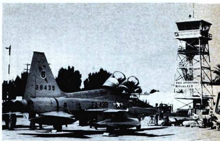
Two-seat version, the F-5B, sits on the ramp at Williams AFB during Tactical Air Command evaluations. Area-ruled tip tanks conform to the aircraft's basic area-rule design. F-5B serves as a trainer and can perform most of the single-seat F-5A missions, but does not have 20-mm. cannons.
