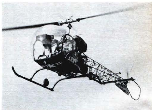
One of the Army's earlier helicopters was the Bell H-13. This machine was a workhorse during the Korean War, serving both as an observation and command vehicle and for the evacuation of wounded. Photo shows the “H” model.
