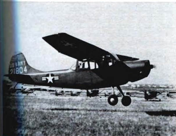
Cessna O-1E liaison and observation plane has been widely used by Army. It's a direct development from the artillery spotters used during World War II. The O-1E now is being replaced by the new light observation helicopters.
