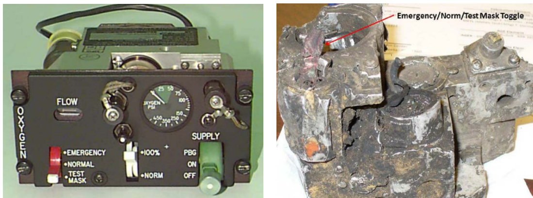
Figure 5: Image of Intact Oxygen Regulator and Image of Damaged Oxygen Regulator from the Mishap Aircraft (Tab J-7 and J-9)
