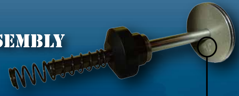
Above: Each of these bi-metal disks slide onto the valve stem assembly with the visible stamped "H" facing out on each disk. The QA shop determined this during an investigation into generator failures. The root of the problem was a technical order, which did not specify the proper configuration. Today the fleet has updated TOs thanks to the efforts of Kingsley Maintainers- most notably the 173rd QA shop.
