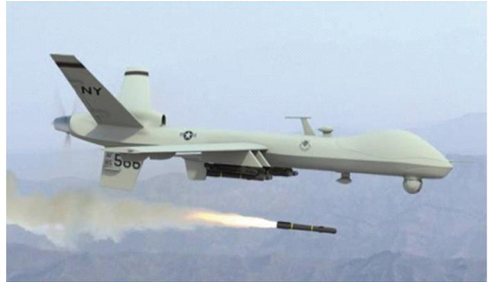
and weapons. C-band line-of-sight datalinks are used for RPA launch and recovery operations, and Ku-band satellite links are used for RPA mission control.
