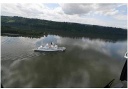
The ship's designation is T-AGM 25 and was built in Pascagoula, Miss., by VT Halter Marine, Inc. It weighs in at 12,642 tons and is 534 feet in length, with a beam of 89 feet.
