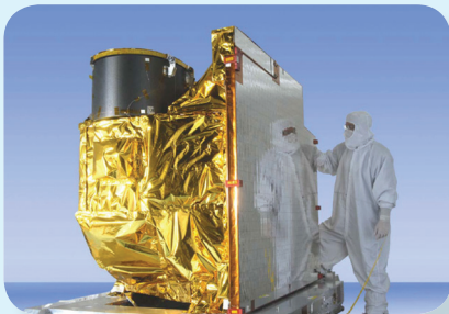
The Advanced Baseline Imager, developed for the GOES-R satellite series, will improve every product the current GOES imager produces and will provide new products that enhance weather forecasting. Credit: NOAA/NASA
