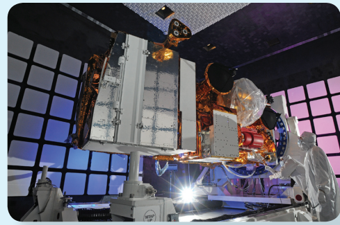
The Suomi NPP satellite underwent electromagnetic interference testing, shown here, in preparation for its October 2011 launch. Credit: NASA
