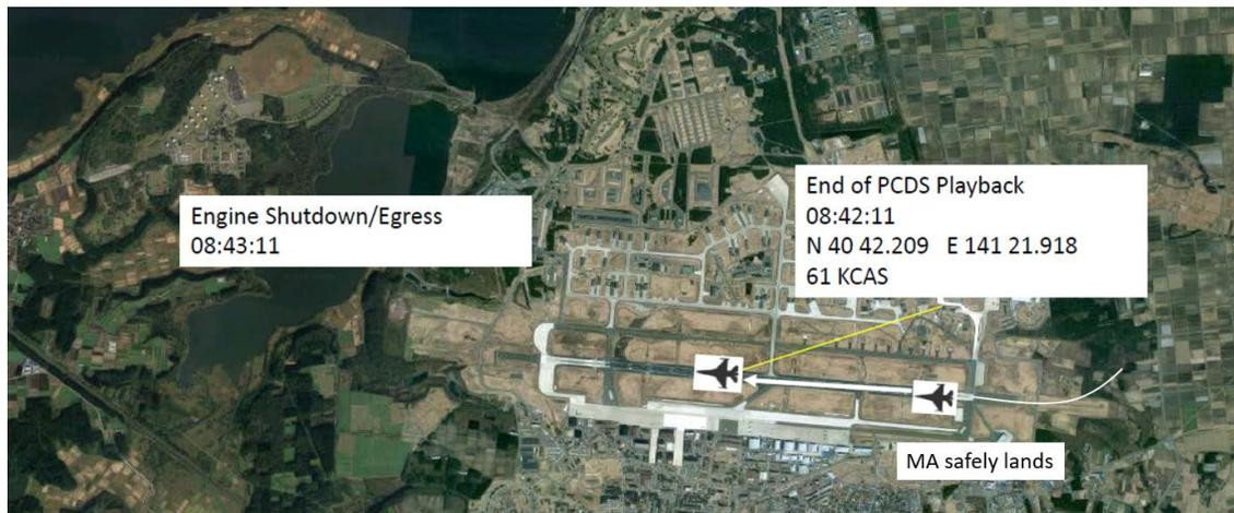
**Figure 3: Mishap Aircraft Mishap Timeline (Tab Z-33)**
