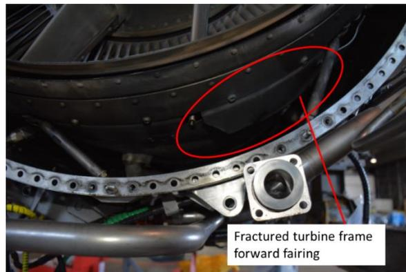
**Figure 6: Turbine frame forward fairing damage at 5:30 position (Tab CC-75)**
