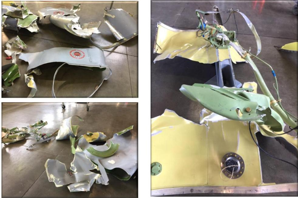
**Figure 20: F-16CM External Fuel Tanks-recovered material from Lake Ogawara**
