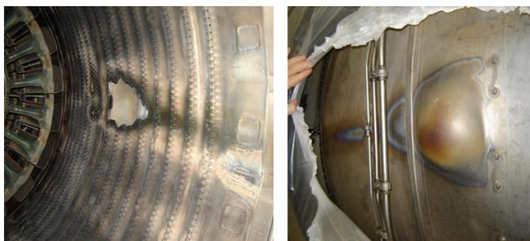
**Figure 18: Exhaust duct liner and duct heat distress from event in 2009 (Tab CC-77)**
