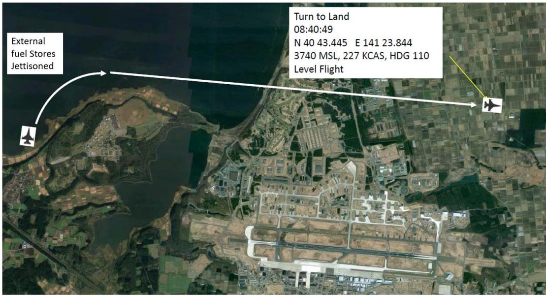
**Figure 2: Mishap Aircraft Mishap Timeline (Tab Z-32)**
