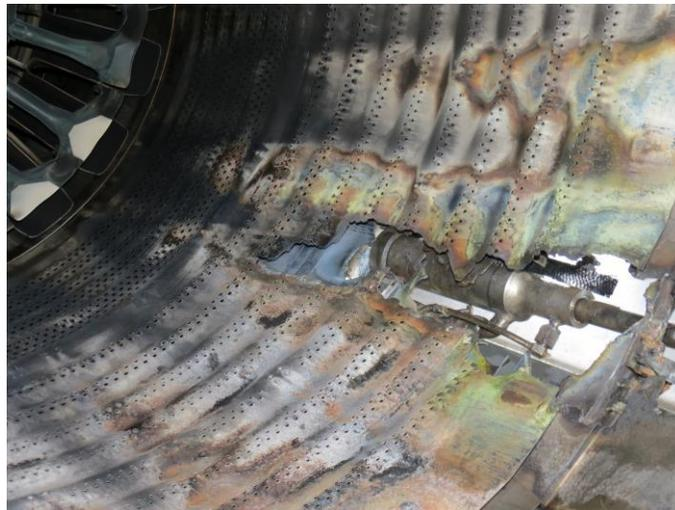
**Figure 16: Burn-through on exhaust duct liner and duct at 4:30 (Tab CC-74)**
