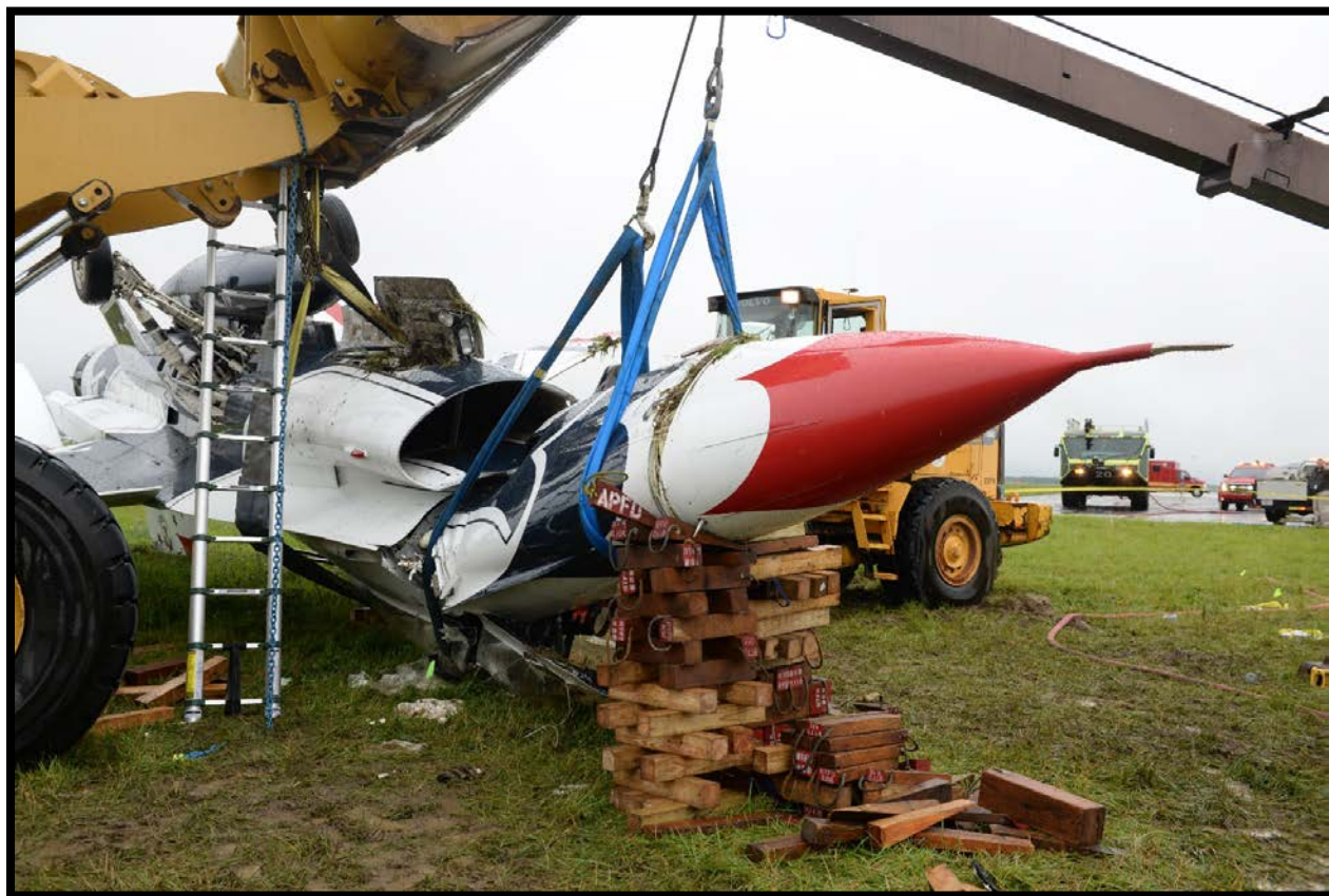
Figure 5. MA stabilized by cribbing and heavy equipment (Tab S-6)
