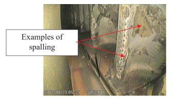
Figure 8: HPT Blades Leading Edge and Platform (Tab J-17)
