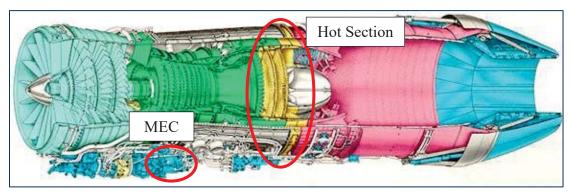
Figure 5: F110-GE-100C Engine Cross Section Overview (Tab J-6)
