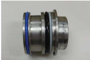
Figure 14: Pressurizing valve transfer tube – Black ring is Viton (Tab J-86)
