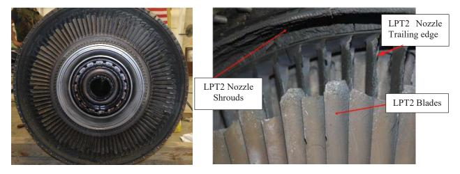
Figure 11: LPT Stage 2 Blades (Tab J-22) Figure 12: LPT Stage 2 Blade Distress (Tab J-23)
