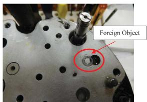
Figure 13: Foreign Object backing ring (Tab J-84)
