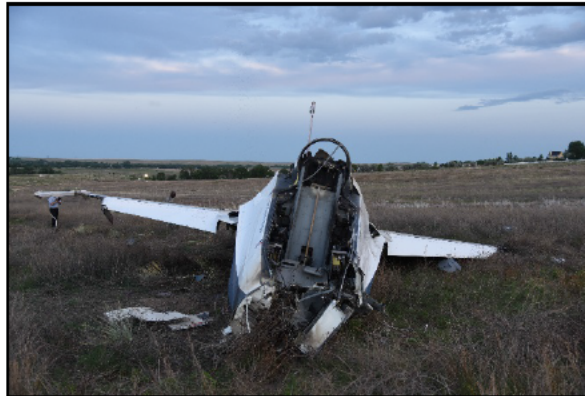
Figure 7. Front view (looking aft) of MA showing damage to cockpit and right and left wings (Tab Z-2)
