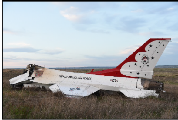
Figure 8. Left view of MA showing partial cockpit separation and damage to tail section of engine bay (Tab Z-3)
