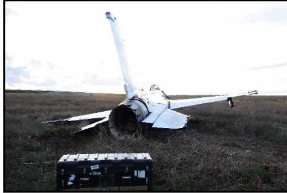
Figure 13. Photo showing damage to MA right horizontal stab, right and left wing tips (Tab Z-9)
