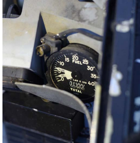
Figure 5. Fuel gauge for the MA indicating approximately 900 pounds of fuel in the fuel tanks after impact (Tab Z-13)
