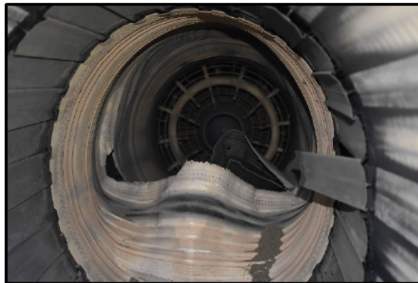
Figure 15. Damage to MA engine exhaust (Tab Z-10)
