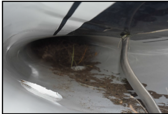
Figure 14. Damage to MA engine intake (Tab Z-5)
