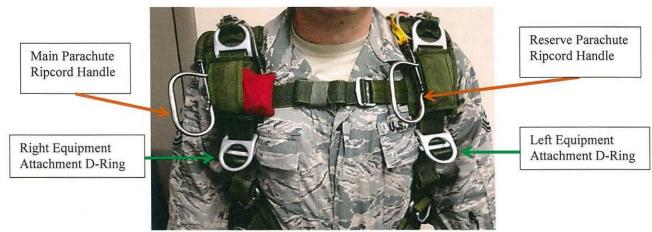
Figure 11.1. Note proximity of the equipment D-rings to the lower portion of the ripcord handles.
