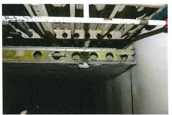
Figure 6.1. Damage to MA's aft cargo door. (Tab S-2)
