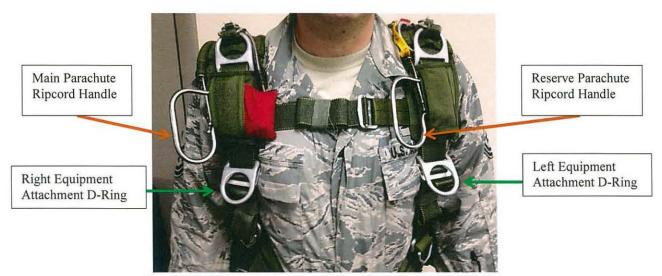
Figure 4.2. MC-4 parachute ripcord handles and equipment D-rings
