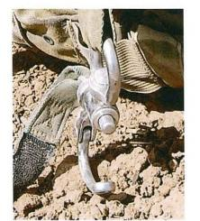
Figure 4.8. Left Quick-Release Shackle (Tab S-6)
