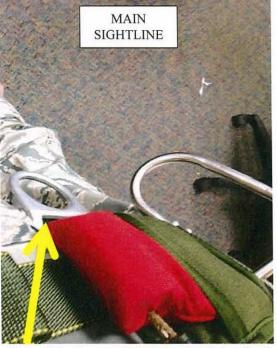
**Figure 11.3.** From a parachutist's point of view (looking down and right) there is space between the main ripcord handle and D-ring. (Yellow arrow indicates sightline)
